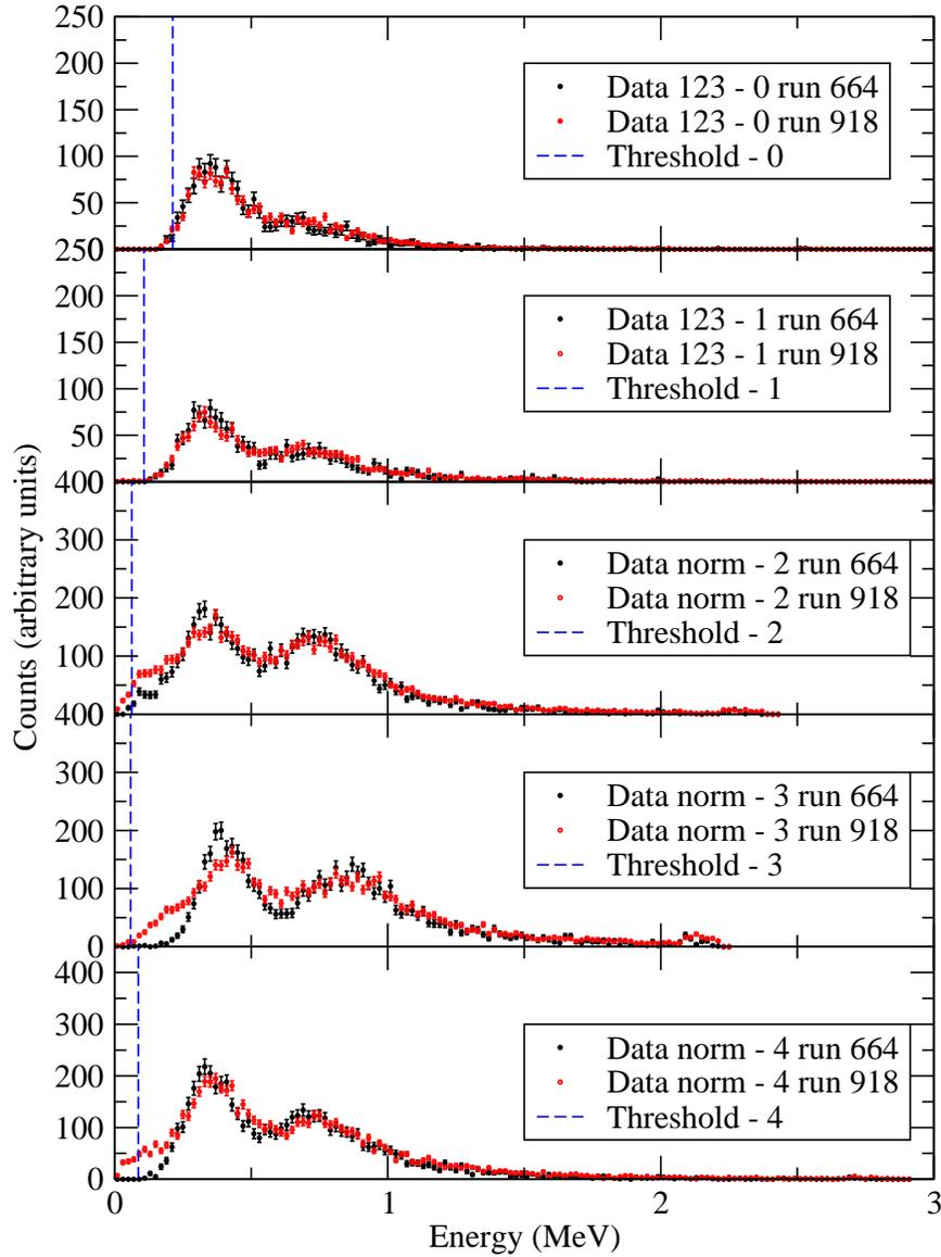
Figure 7: The spectra taken different photon rates. Run 664 is at a very low rate while run 918 is at a rate of about  $9 \times 10^6$  Hz.
