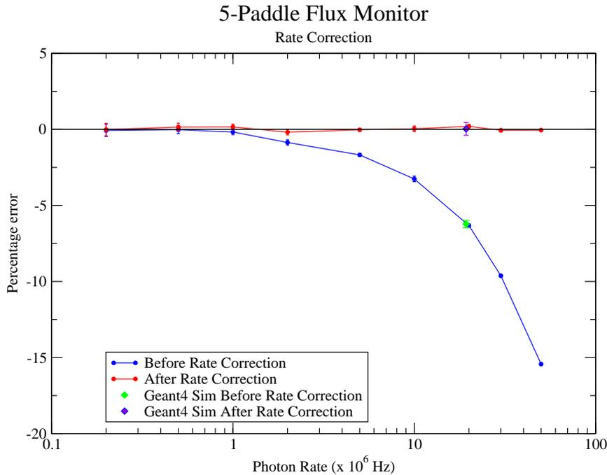
Figure 6: The percentage error in the number of photons as a function of photon rate. The errors without applying a rate correction and after applying a correction are shown.
