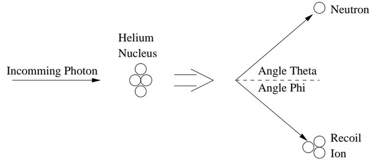
Figure 1: The reaction  ${}^4\text{He}(\gamma, n){}^3\text{He}$
