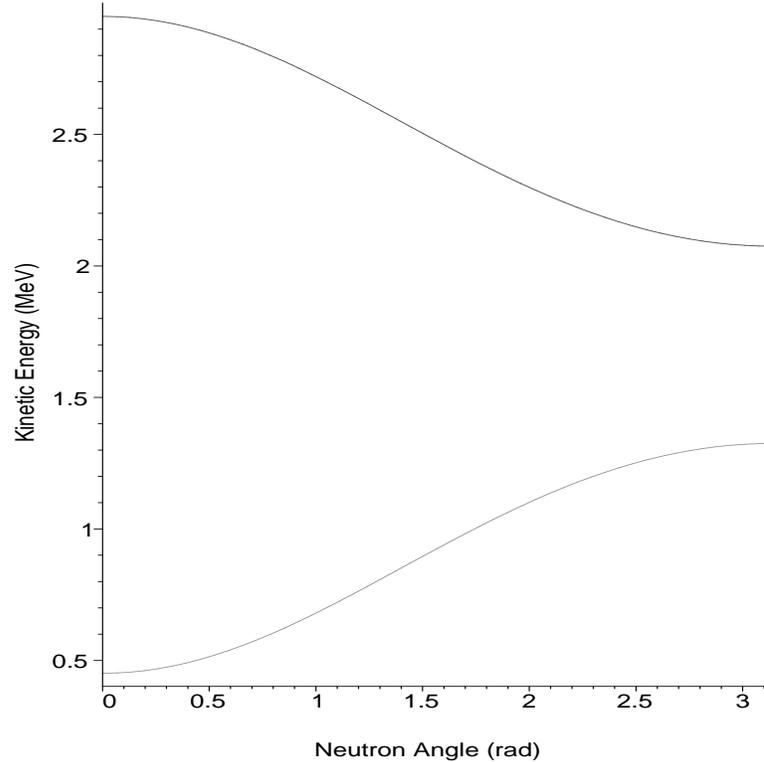
Figure 2: The kinetic energy of the neutron (top) and  ${}^3\text{He}$  ion (bottom) emitted from a  ${}^4\text{He}(\gamma, n){}^3\text{He}$  reaction with  $E_\gamma = 24$  MeV
