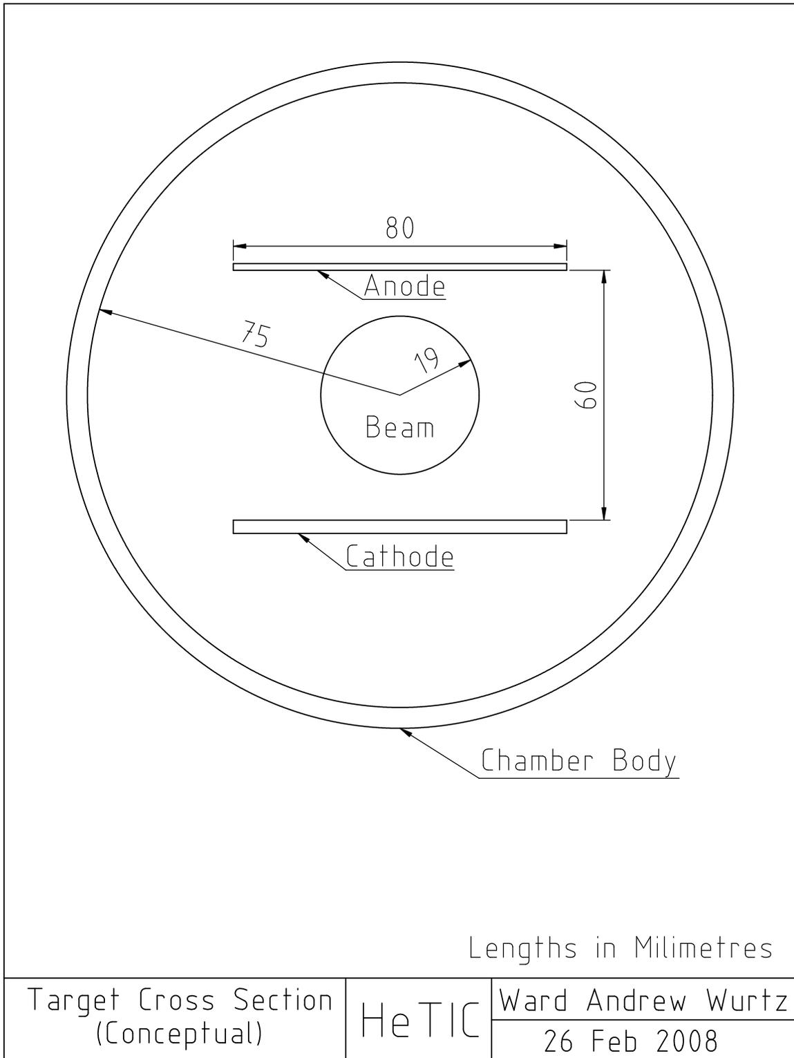
Figure 6: HeTIC cross section conceptual diagram
