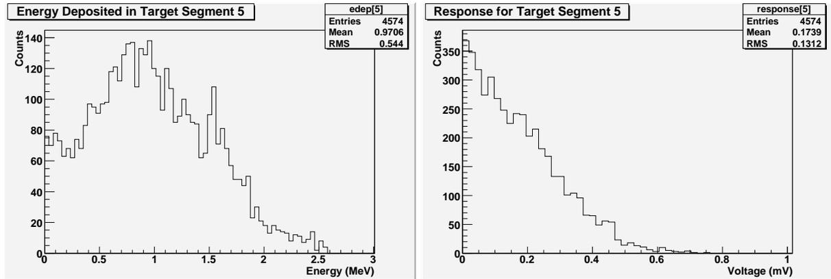
Figure 11: The energy deposited and response histograms for  $^3\text{He}$  ions produced from photodisintegration reactions caused by 30 MeV photons in a 3.8 cm diameter beam
