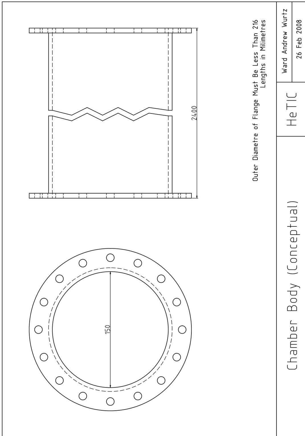
Figure 7: HeTIC chamber body conceptual diagram
