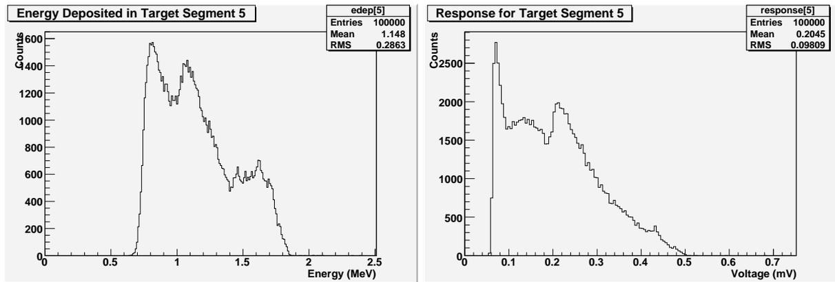
Figure 10: The energy deposited and response histograms for  $^3\text{He}$  ions produced from photodisintegration reactions caused by 30 MeV photons in the centre of a target segment
