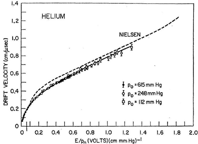
Figure 4: The electron drift velocity of Bowe (points, solid line) and Nielsen (dashed line) from figure 4 of [Bowe]
