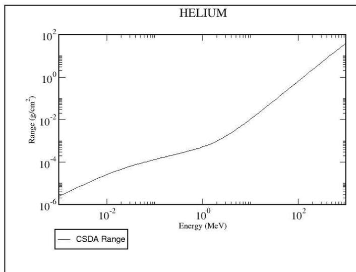
Figure 3: The range of an alpha particle in helium from [BCZC]
