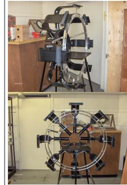
At the end of the summer all of the aforementioned components of the cosmic ray detector were assembled together and working properly. A stand to support the detectors was constructed as well as a circuit box to house the circuitry. The detector array is intended to be put on display in the physics building's foyer for the general public
