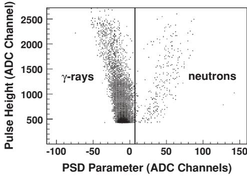
FIG. 2. A PSD spectrum with the applied cut indicated by the vertical line. These data are taken from a single detector over the course of a single 1-h runs.
