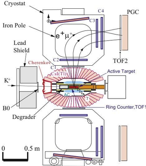
**Fig. 1.** Cross-sectional side views of the setup for the J-PARC E36 experiment [2,3]. The momentum vectors of charged particles and photons are determined by the toroidal spectrometer and the CsI(Tl) calorimeter, respectively. The spectrometer has 12 identical gaps and a rotational symmetry of  $30^\circ$ . Charged particles will be discriminated by a combination of measurements from the PGC, AC, and TOF detectors. The PGC is located at the end of the detector system.
