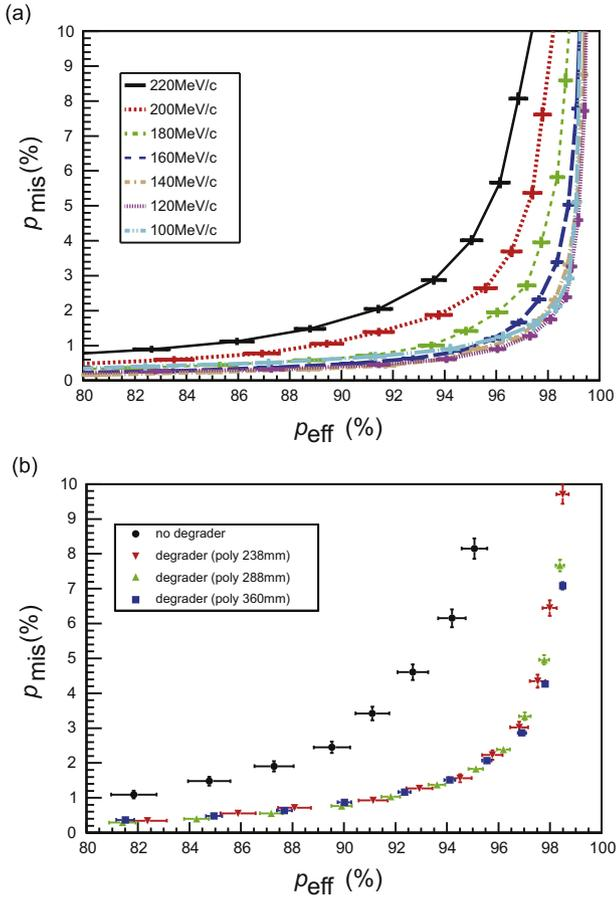
**Fig. 6.** Correlation plots of  $\mu^+$  mis-identification probability and  $e^+$  efficiency obtained by changing (a) the initial beam momentum and (b) the degrader thickness using a 240 MeV/c incident beam. The detector performance is highly improved by decreasing the incident beam momentum. Using a polyethylene degrader, we succeeded in reducing the muon mis-identification probability down to 5% with keeping the high  $e^+$  efficiency of 98%.
