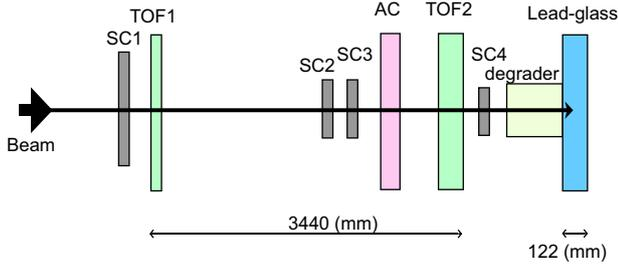
**Fig. 3.** A schematic view of the beam test setup at TRIUMF M11. We injected a mixture of  $e^+$ ,  $\mu^+$ , and  $\pi^+$  beams with momentum from 100 to 240 MeV/c. The TOF system and the AC counter placed upstream of the lead-glass blocks were used for particle identification in the analysis. The polyethylene degraders were placed in front of the lead-glass blocks to decrease the beam momentum.
