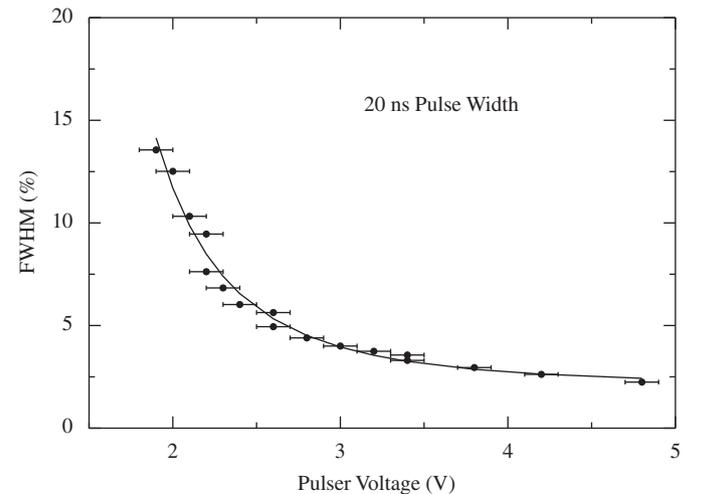
Fig. 3. The measured FWHM of the light output of the NSPB310 LED as a function of pulser voltage for a pulse width of 20 ns. The line is a fit to the data points.
