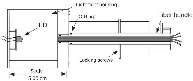
**Fig. 4.** A schematic of the light tight LED housing which mates to the end of a bundle of optical fibers.
