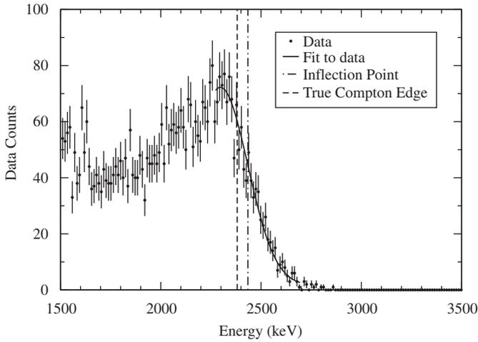
**Fig. 6.** An example of fitting to the Compton edge in a BC-505 cell. The data points with error bars shows the Compton edge for the 2.614 MeV gamma ray from a thorium source. The solid line shows the fit to the data used to find the inflection point which is shown by the vertical dot-dashed line. The energy scale has been calibrated so that the position of the inflection point matches that determined from a simulation. The vertical dashed line shows the energy of the Compton edge.
