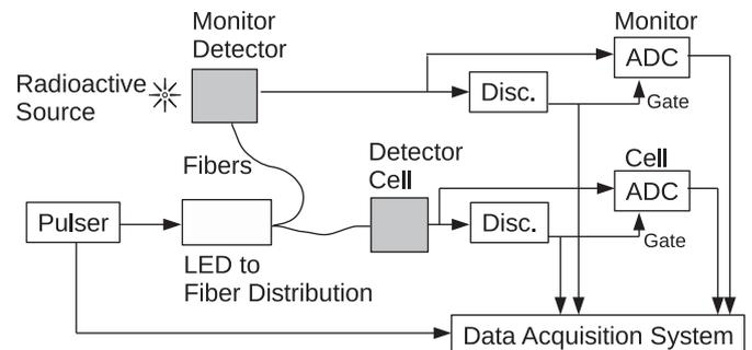
Fig. 2. Conceptual schematic of the gain monitoring system. When the pulser fires the data acquisition system will record ADC values from the detector cells as well as from the monitor detector. In addition, the data acquisition system will record ADC values from the monitor detector when a signal caused by the radioactive source is present and the pulser is not present.
