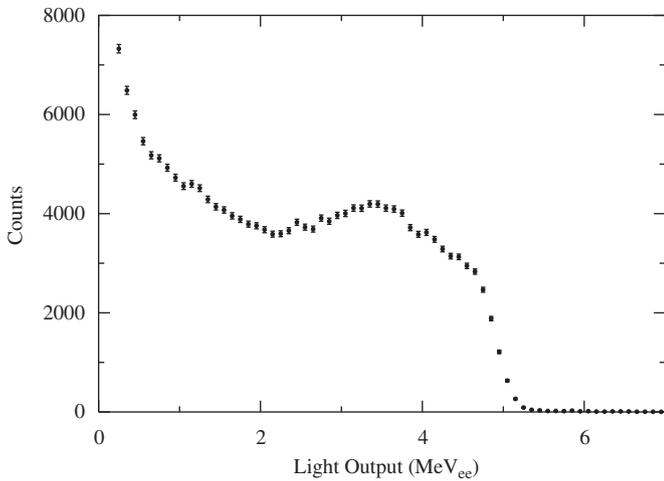
Fig. 1. The spectrum from a BC-505 scintillator cell when 8.78-MeV neutrons are incident on it. The spectrum was generated by a GEANT4 simulation.
