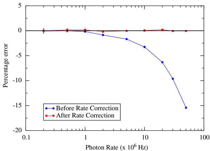
**Fig. 8.** The percentage error in the number of photons as a function of photon rate. The errors without applying a rate correction and after applying a correction are shown. Uncertainties in the simulation results are smaller than the size of the data points shown.
