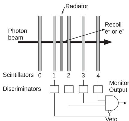
Fig. 1. Conceptual design of the photon flux monitor.
