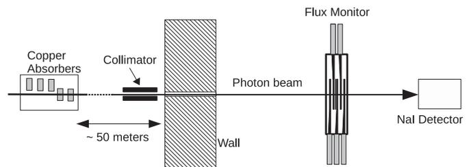
**Fig. 5.** A schematic of the experimental arrangement used to characterize the photon flux monitor (not to scale).
