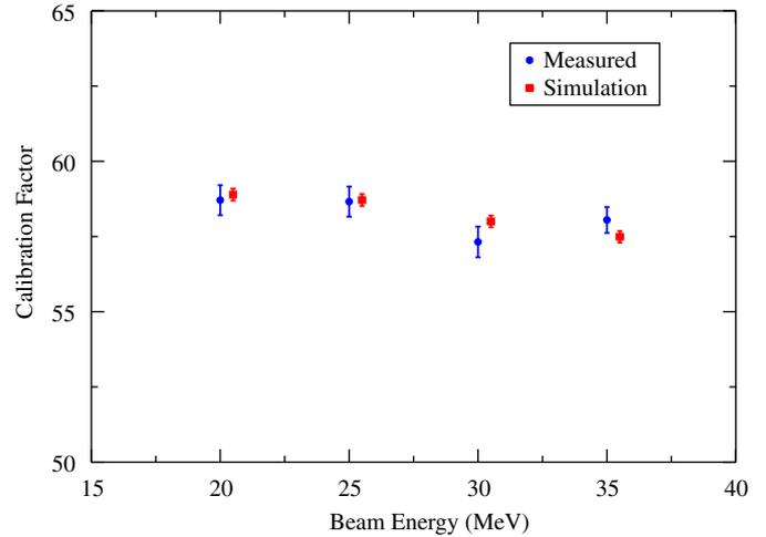
**Fig. 7.** Measured calibration factors and calculated calibration factors for the five-paddle flux monitor as a function of energy. For clarity the simulated values are offset by 0.5 MeV from the measured data points.
