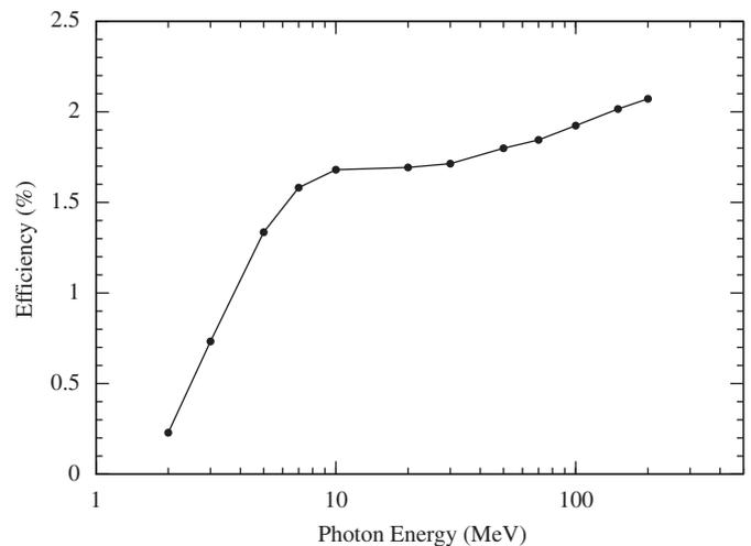
Fig. 2. The efficiency of the flux monitor, as calculated using the GEANT4 simulation, is plotted as a function of photon energy. The uncertainties in the calculated points are smaller than the plot symbols.
