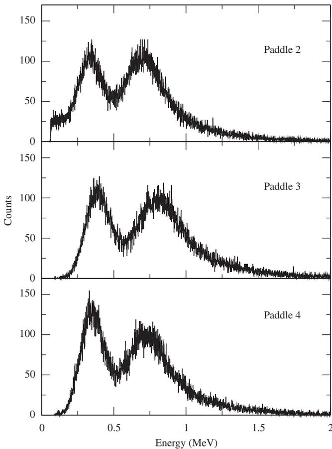
**Fig. 3.** Paddle spectra calculated from the simulation for a photon energy of 30 MeV. The spectra shown are for the condition of a triple coincidence between paddles 2, 3 and 4 and no hit in the veto paddle 1. Note that the energies of the minimum ionizing peaks for each paddle are at slightly different energies since the paddles have slightly different thicknesses.
