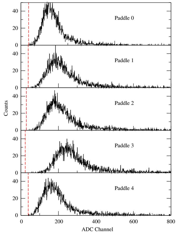
**Fig. 4.** The measured spectra from the five paddles due to cosmic ray muons when a coincidence between all five is required. Dashed lines show the threshold for each paddle.
